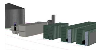
Why is biogas the optimal technology in this situation?: The gas will be fed to an on-site CHP unit, to supply 110kW hours of power to the site and up to 90 kW of heat.
