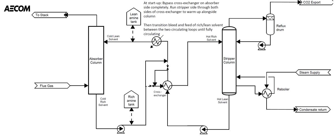
AECOM (2020) for BEIS, Start-up and Shut-down times of Power CCUS Facilities.
