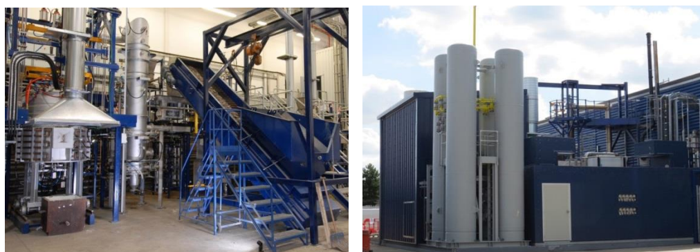
Figure A-3: The major components of the pilot plant: two-stage fluidised bed and plasma converter for syngas generation (left), syngas storage vessels and BioSNG facility (right)
