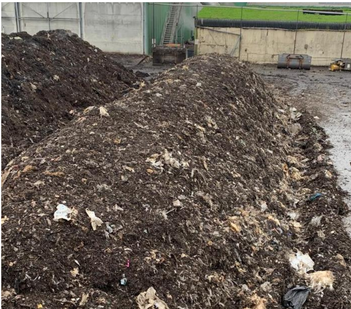
Figure 5 -The segregated windrow, containing the compostable test materials/ packaging was placed at the end of "Row 1, Old Pad". This row has just been mechanically turned. The profile is a roughly rounded trapezoid.
