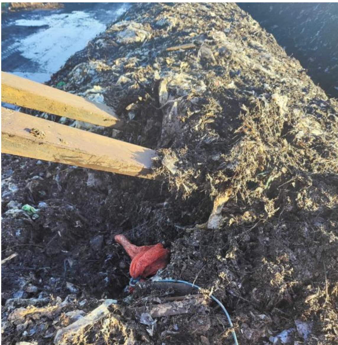
Figure 9 - Sample being buried in the material using a forklift truck to easily make a hole in the pile showing the bag being set at an estimated 1m deep.
