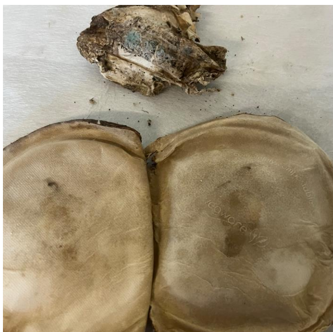
Figure 15 – SAMPLE 8 after tunnel phase of composting, found to be stacked together which clearly reduced break down rate.
