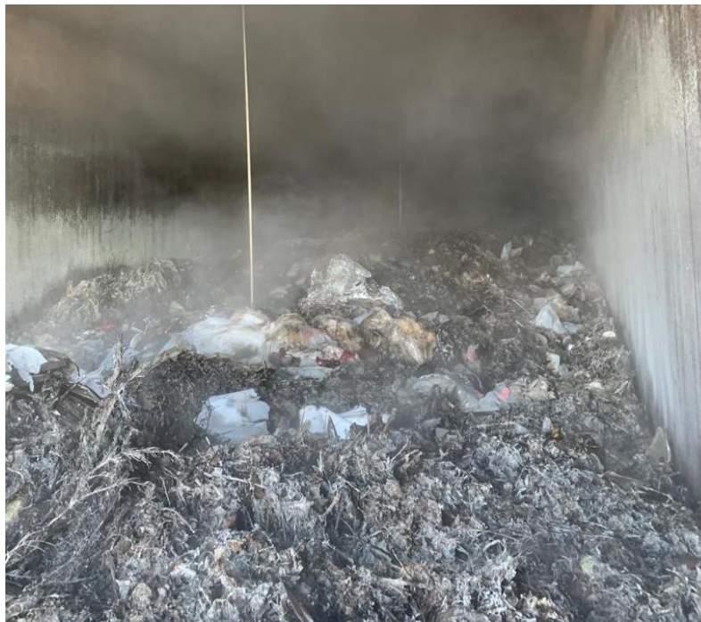
Figure 3 - Material in the composting tunnel being processed between Christmas and New Year 2022. 50% through its allotted time in the IVC tunnel.
