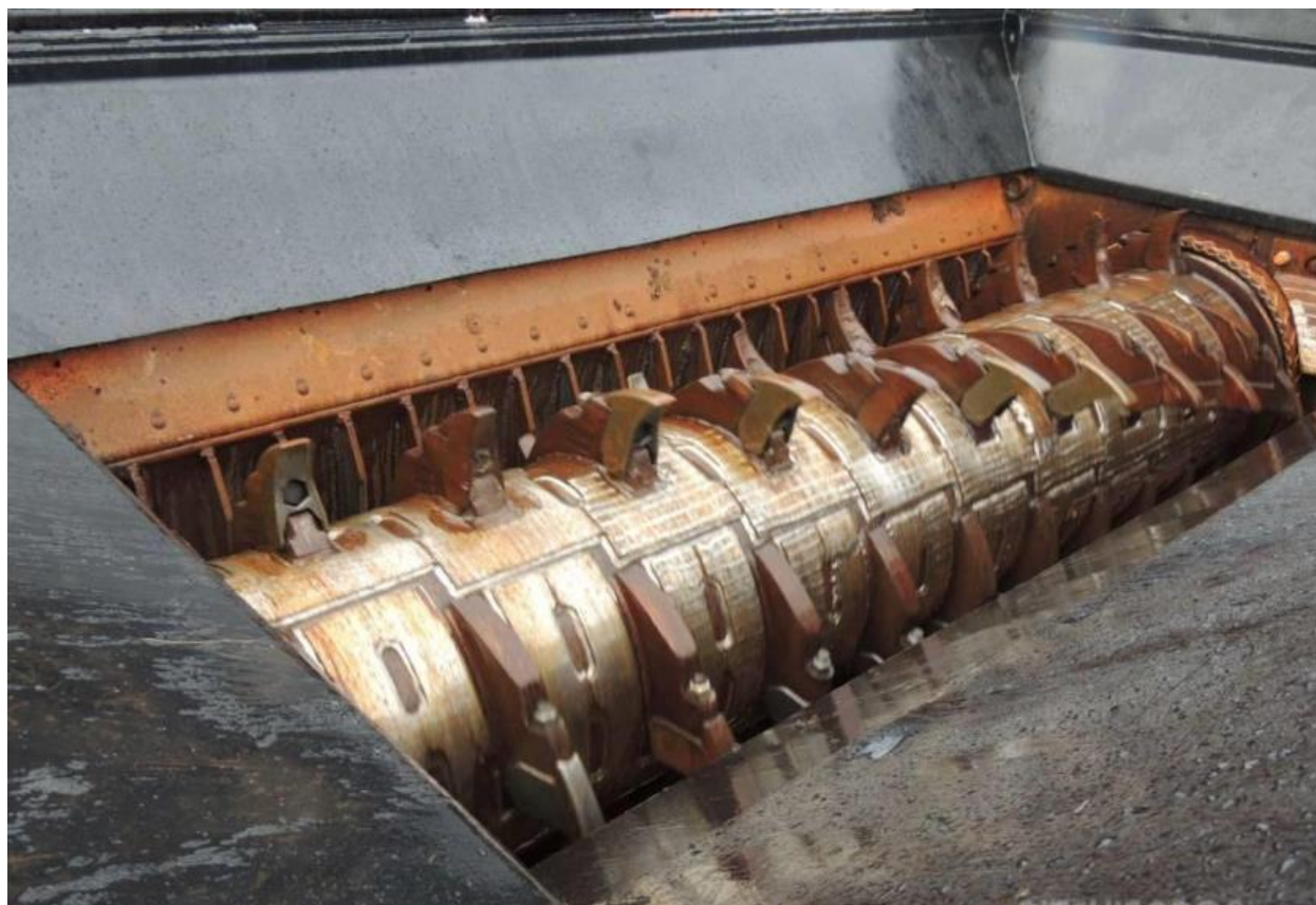
Figure 2- The shredding rotor on a Doppstadt 3060 Biopower - showing teeth and rake configuration. There is a further rake, which the teeth move through deeper into the machine.
