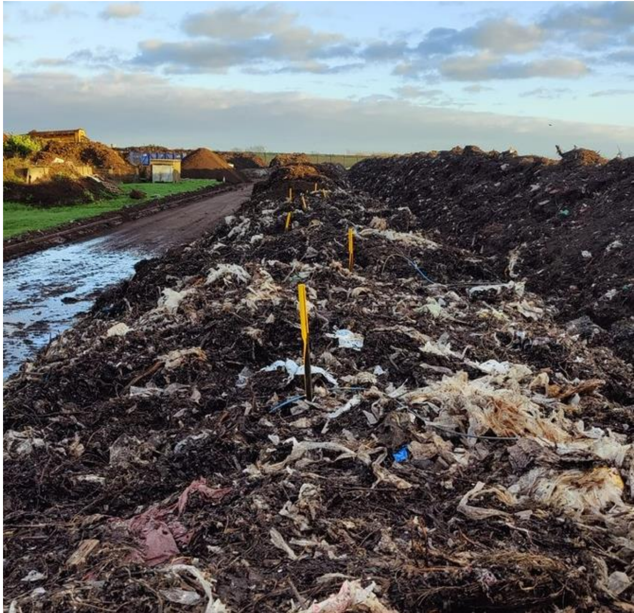
Figure 8 - Composting windrow with markers showing the location of the sample mesh bags required for analysis during composting process.
