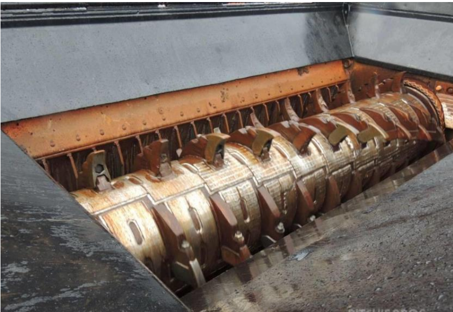
Figure 1 – Samples were shredded using a Doppstadt 3060 biopower industrial shredder, shred to a maximum of 400mm in any one plane.
