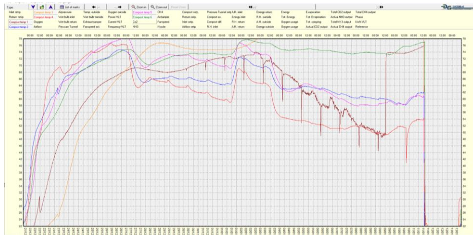
Figure 2 – Time temperature data from the computer. The controlled SCADA systems use process feedback to adjust the composting parameters, ensuring optimum composting conditions are maintained.
